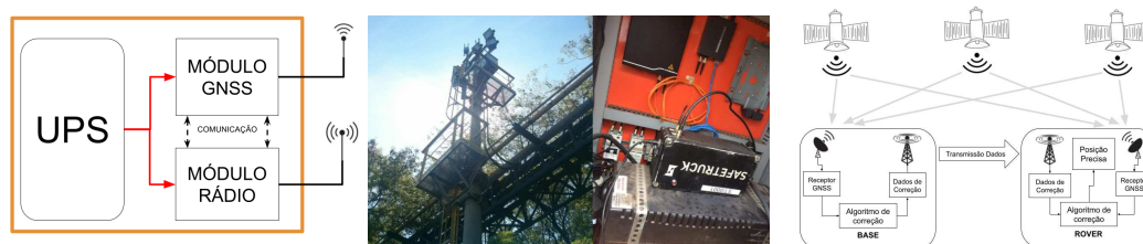
Figure 1. Block diagram of the base station used in the POC and installation, and RTK correction system.
