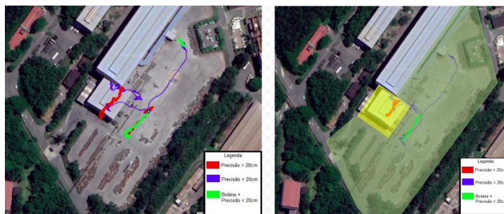
Figure 5. Tracking while moving between control points and continuous precision analysis.
