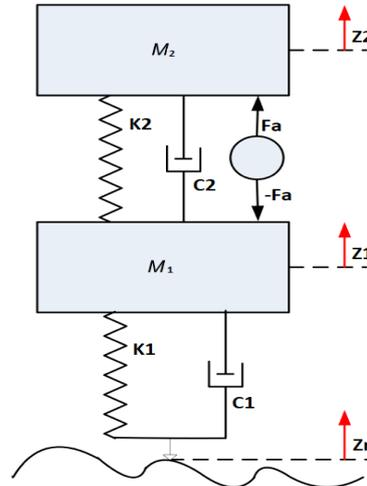
Figure 1. ¼ Car suspension model. Available from: QUANSER MANUAL, 2010
