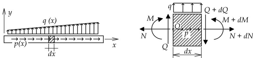
Figure 2. Timoshenko beam displacement field (Rodrigues et al. [4])
