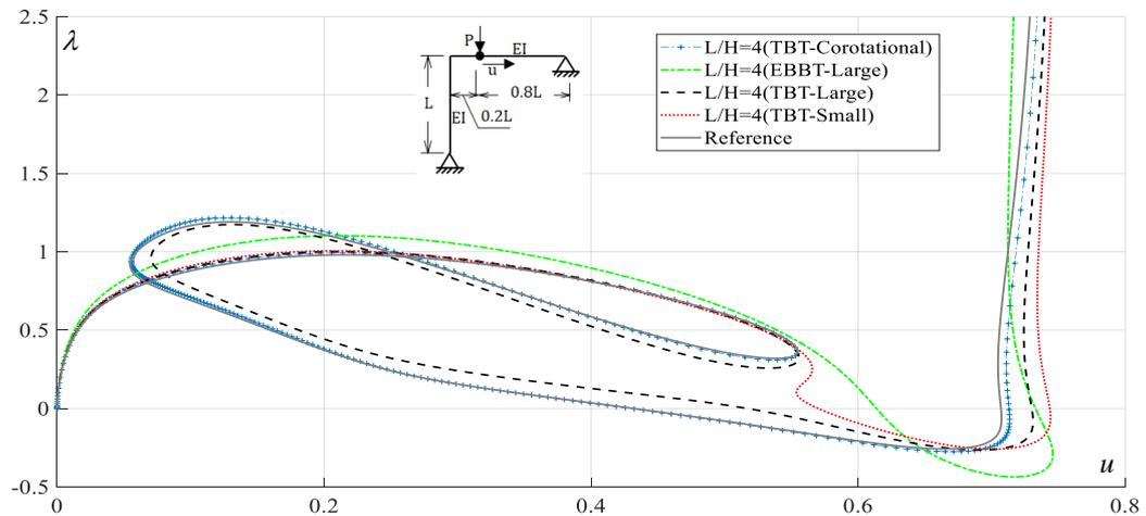
Figure 9. Lee frame equilibrium path for 5 elements in each bar -  $L/h = 4$
