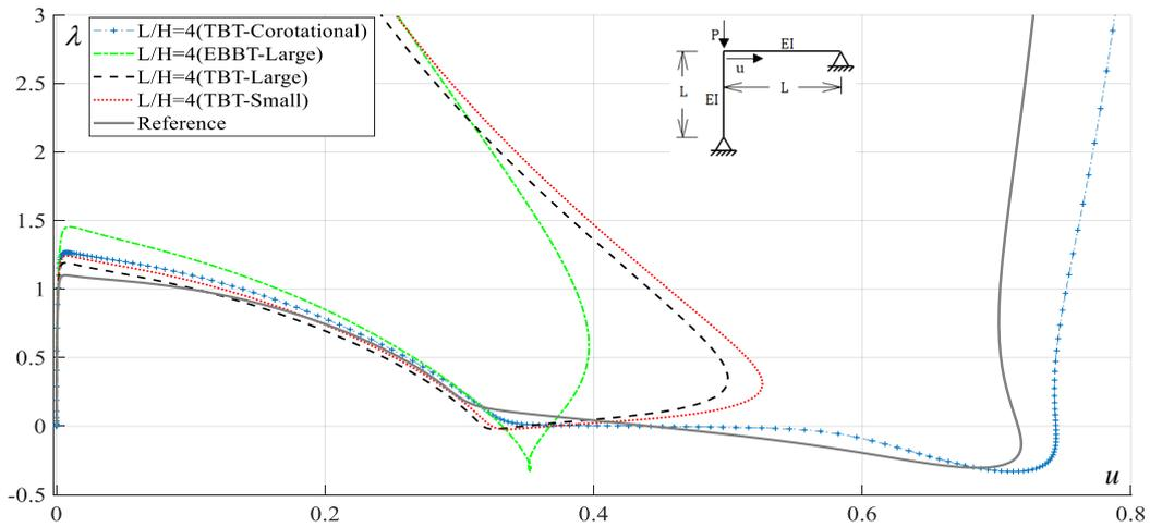
Figure 7. Roorda frame equilibrium paths for 2 elements in each bar -  $L/h = 4$
