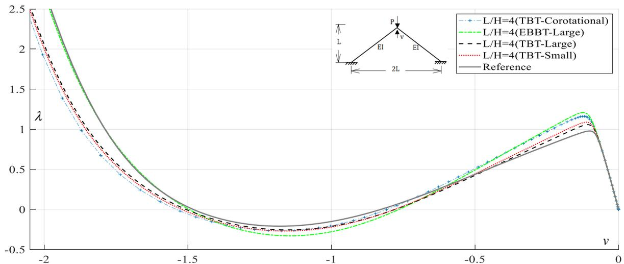
Figure 5. Toggle frame equilibrium paths for 2 elements in each bar -  $L/h = 4$
