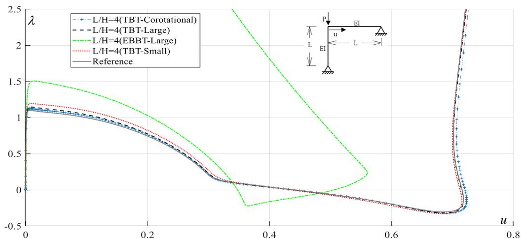
Figure 8. Roorda frame equilibrium paths for 5 elements in each bar -  $L/h = 4$
