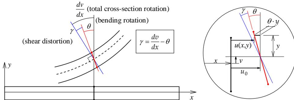
Figure 1. Timoshenko beam displacement field (Rodrigues et al. [5])
