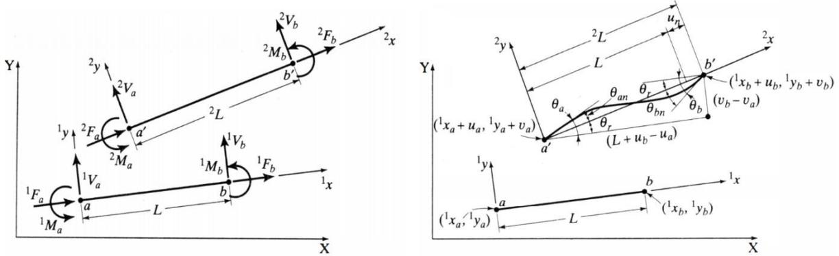
Figure 3. Element forces and displacements (McGuire et al. [1])
