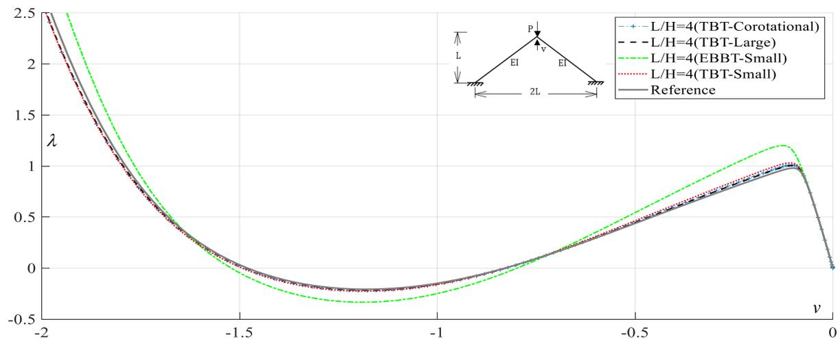
Figure 6. Toggle frame equilibrium paths for 5 elements in each bar -  $L/h = 4$
