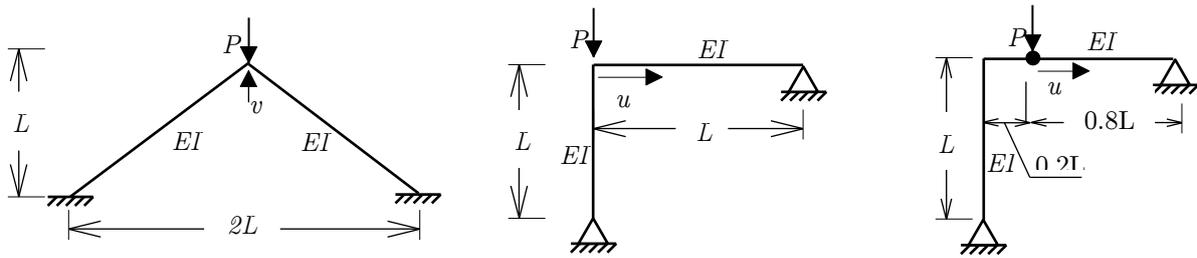
Figure 4. (a) Toggle frame, (b) Roorda frame, (c) Lee frame
