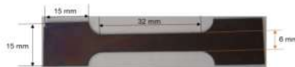
Figure 4 - Tensile test specimen
