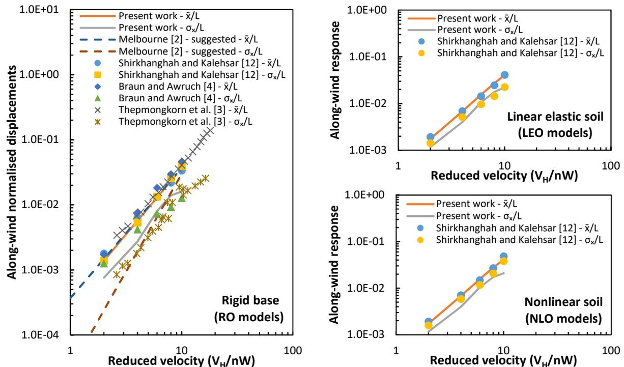
Figure 6. Along-wind normalized displacements as functions of the wind reduced velocity
