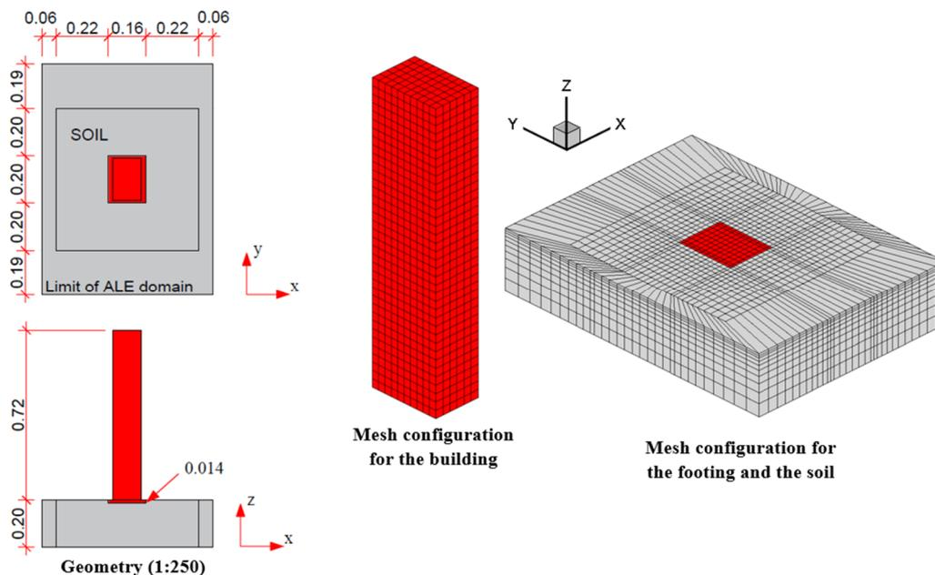
Figure 5. Geometrical characteristics and mesh configuration used for the aeroelastic analysis of the CAARC building model
