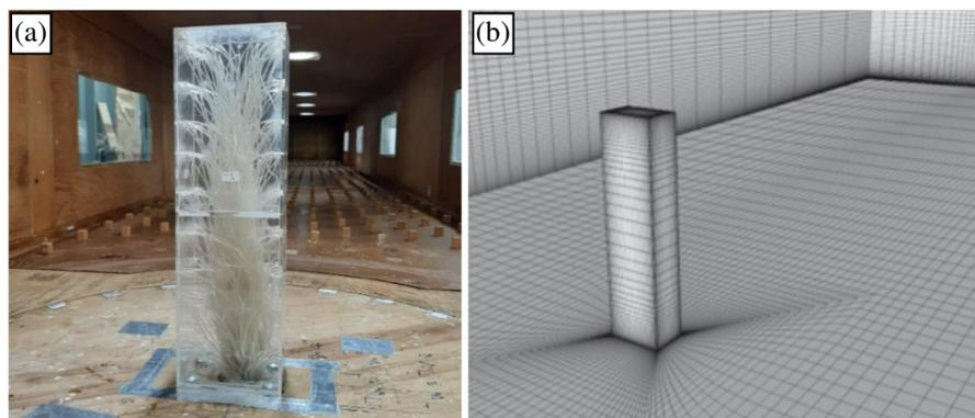
Figure 1. Aerodynamic analysis of the CAARC building: (a) experimental model by Fontes-Silva et al. [8] and (b) numerical model by Braun and Awruch [4]
