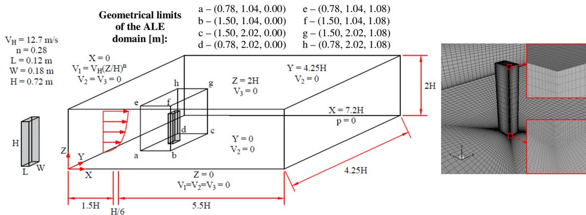
Figure 2. Geometrical characteristics and boundary conditions defined for the CAARC building analysis
