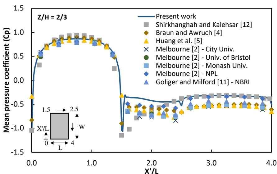
Figure 3. Mean pressure coefficients at  $Z/H = 2/3$  for the CAARC building model
