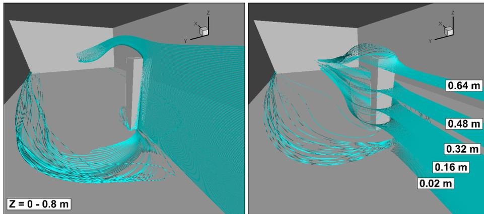
Figure 4. Three-dimensional streamlines obtained from the mean flow field for the CAARC building model
