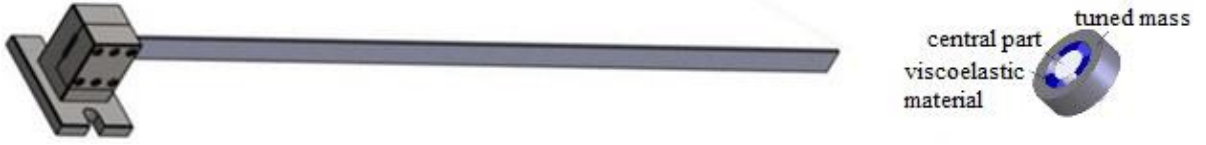
Figure 2. Computational representation of the primary system and of an instance of VDN.
