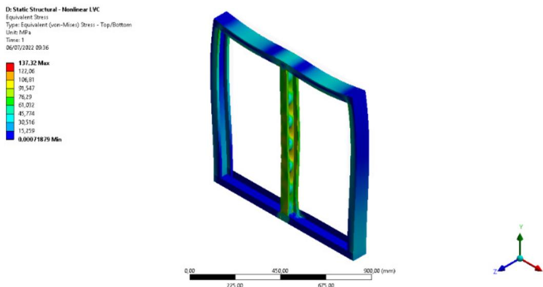
Figure 4. Deformed condition and Von-Mises stresses obtained by analysis 2
