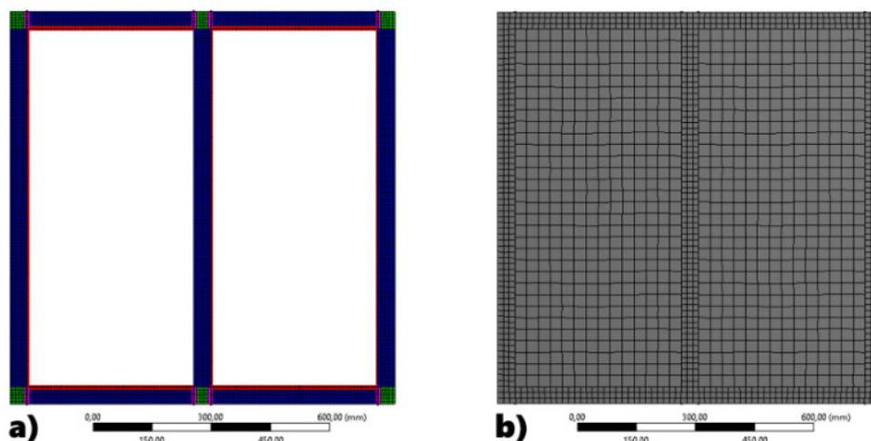
Figure 2a: Internal structure in plate elements, Figure 2b: Gypsum in solid elements
