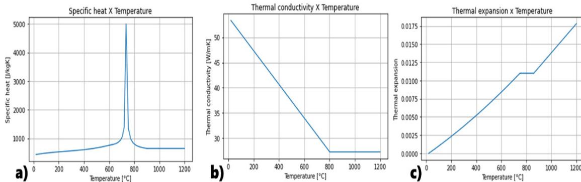
Figure 5a. Specific heat. Figure 5b. Thermal conductivity. Figure 5c. Thermal expansion
