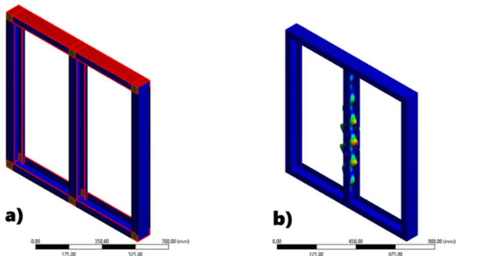
Figure 3a: Structure submitted for analysis 1, Figure 3b: Mode of instability acting on the structure
