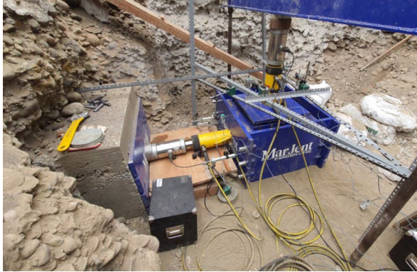
Figure 9.- In situ large-scale direct shear test, conducted by MarJent (October, 2020).
