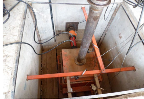
Figure 10.- In situ large-scale direct shear test, conducted by CISMID-UNI (September, 2020).
