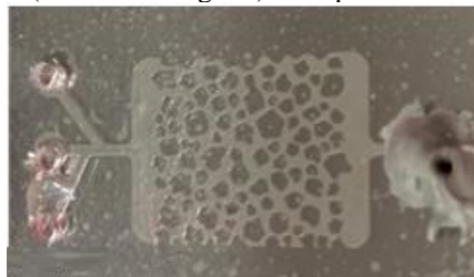
Figure 3. Micromodel made of glass and sealed with NOA81.
