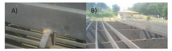
Figure 1. A) Pass-through crack between the front vertical bars and the rack panel tray; B) Failure caused by cracks, with subsequent removal of the vertical bars.
