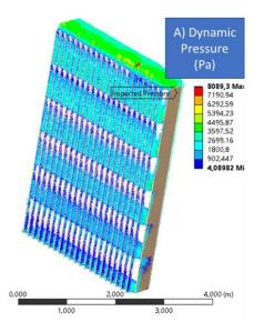
Figure 5. Dynamic pressure (Pa) passed to the structural model. Result obtained from CFD.
