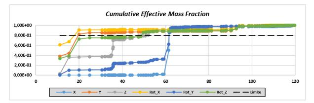
Figure 6. Plot summarizing the various natural frequencies of the structure (abscissa) and the ratio of the effective mass of each mode to the total mass of the structure (ordinate).
