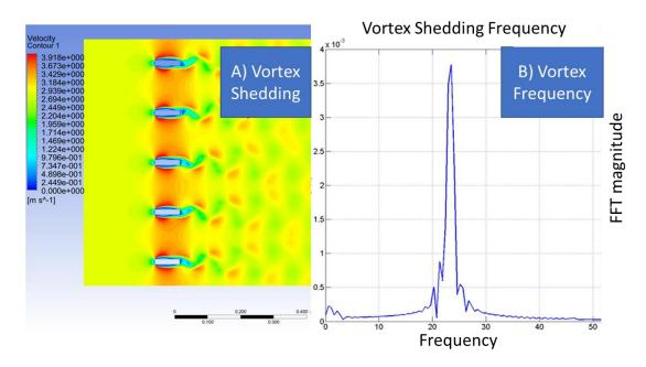
Figure 4. Velocity field (A) demonstrating the existence of alternating vortices and (B) the characteristic frequency of vortex shedding using FFT.
