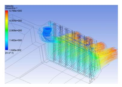
Figure 3. Streamlines (color map as a function of velocity) of water flowing through the grid panels to the penstock.
