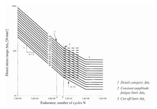
Figure 8. Direct stress range (MPa) as presented in Eurocode 3 for typical cases of welded joints.
