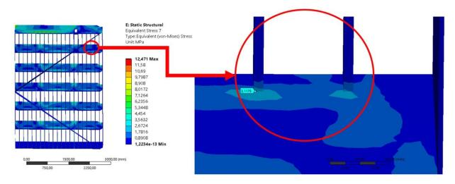
Figure 7. Result (mechanical stress) obtained by applying a weight force to the panel installed on the base plate. Partial result, prior to superposition with the stresses obtained by harmonic loading analysis.
