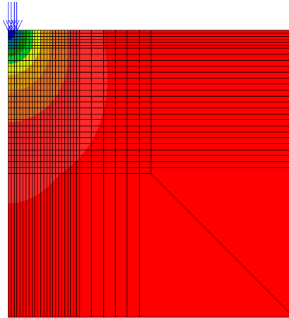
Figure 1. Axisymmetric mesh used for backcalculation.
