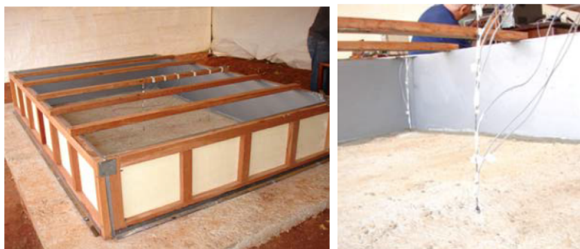
Figure 2. Slab shape tested and monitoring thermometers coupled to the LYNX platform (COPPE/FURNAS).
