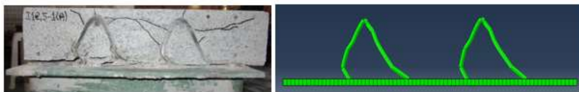
Figure 4. Deformed by the experimental Barbosa connector [1] and deformed by the numerical model
