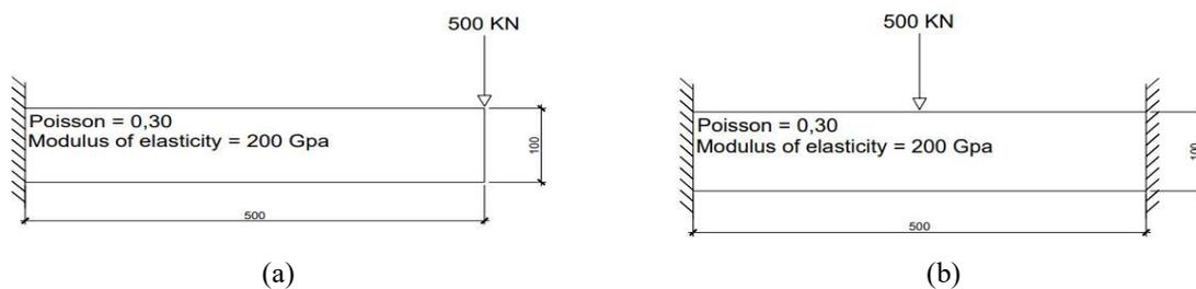
Figure 2 - Beam models: a) Simply supported and cantilever; b) Double-supported.
