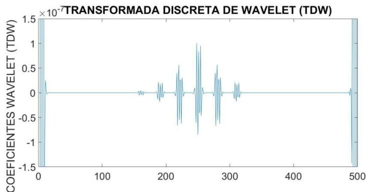
**Figure 6 - Wavelet Coefficient for the double-supported beam.**
