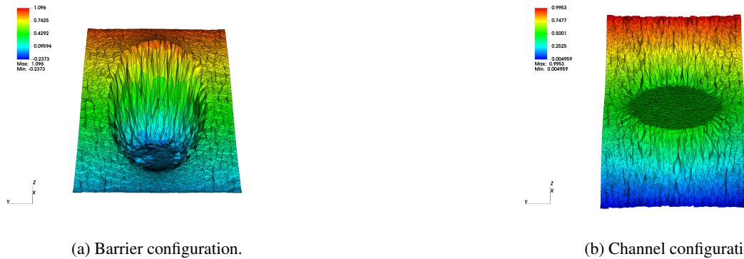
Figure 3. Fine-scale reference solutions for the single-phase simulation of a reservoir containing a spherical heterogeneity under a barrier (a) and channel (b) configuration. Slice at y = 0 .
