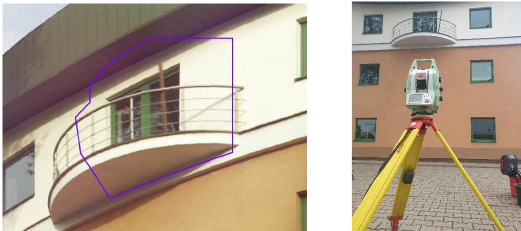
Figure 1. Laboratory tests; from the left: scan area as indicated on the display; from the right: Scanning Total Station during field survey.
