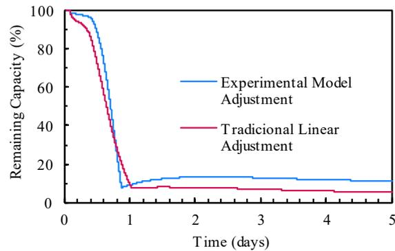
Figure 11. Remaining Capacity (Mohr-Coulomb) x Time (days).
