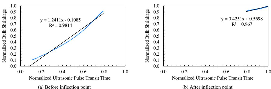
Figure 6. Normalized Bulk Shrinkage x Normalized Ultrasonic Pulse Transit Time.
