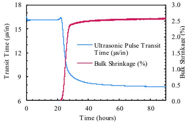
Figure 3. Ultrasonic Pulse Transit Time ( $\mu\text{s/in}$ ) and Bulk Shrinkage (%) x Time (h).
