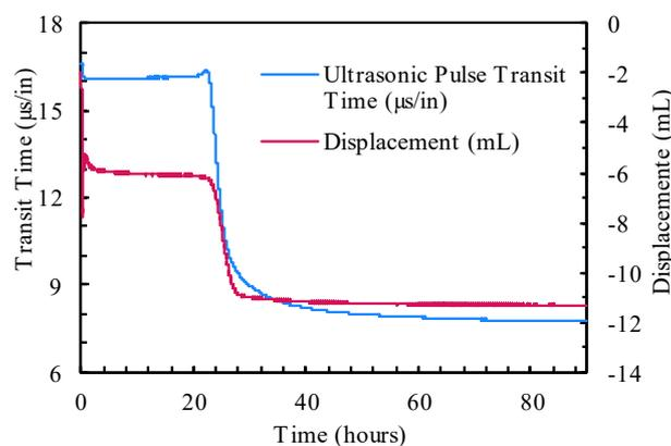
Figure 2. Ultrasonic Pulse Transit Time ( $\mu\text{s/in}$ ) and Displacement (mL) x Time (h).
