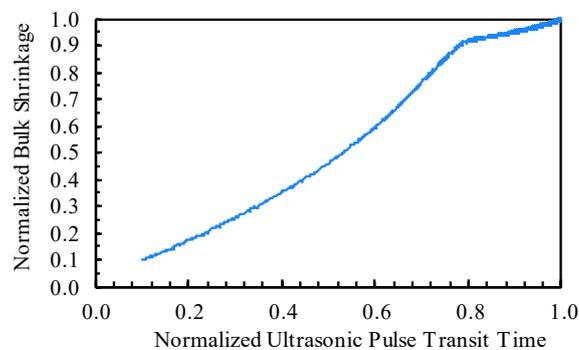
Figure 5. Normalized Bulk Shrinkage x Normalized Ultrasonic Pulse Transit Time.
