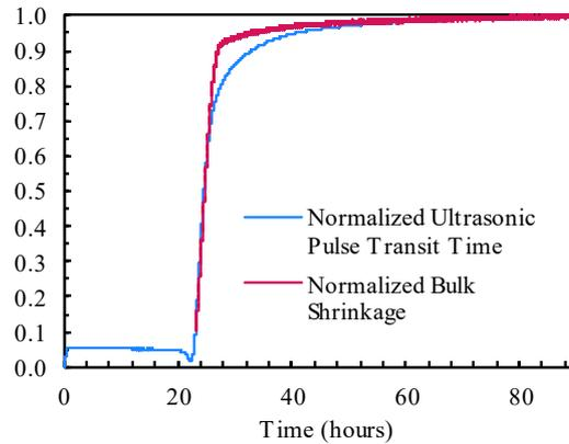
Figure 4. Normalized Ultrasonic Pulse Transit Time and Bulk Shrinkage x Time (h).
