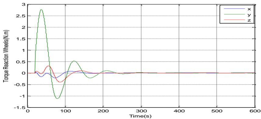
Fig. 5 - SDRE controller using torque due to the reaction wheel.
