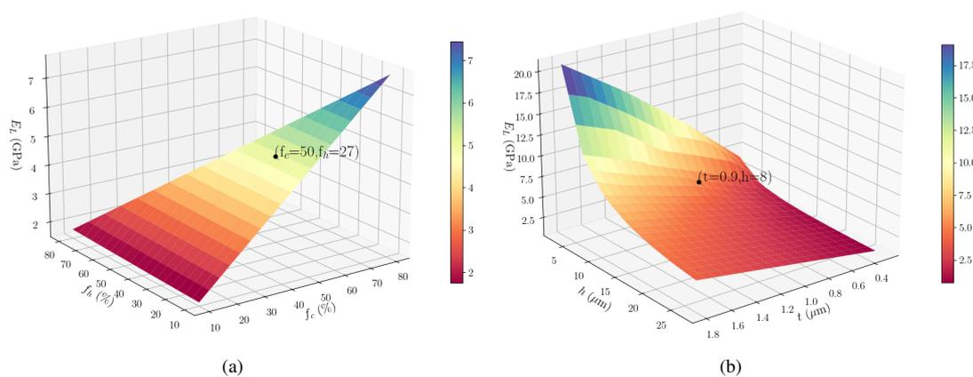
Figure 3. Longitudinal Young's modulus variation with parameters: (a)  $f_c$  and  $f_h$ . (b)  $h$  and  $t$ .
