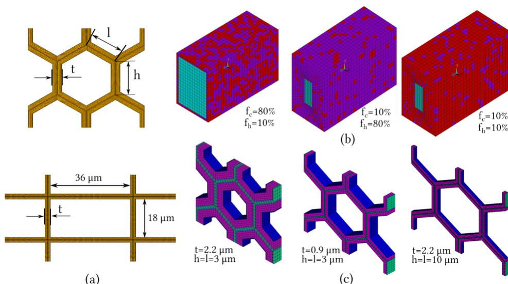
Figure 2. RVE variations for the sensitivity analysis. (a) Geometrical parameters at the meso-scale. (b) RVEs with different values of  $f_c$  and  $f_h$ . (c) RVEs with different  $t$  and  $h$  combinations
