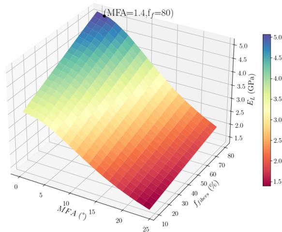
Figure 4. Longitudinal Young's modulus variation with parameters MFA and  $f_f$  at the macro scale.
