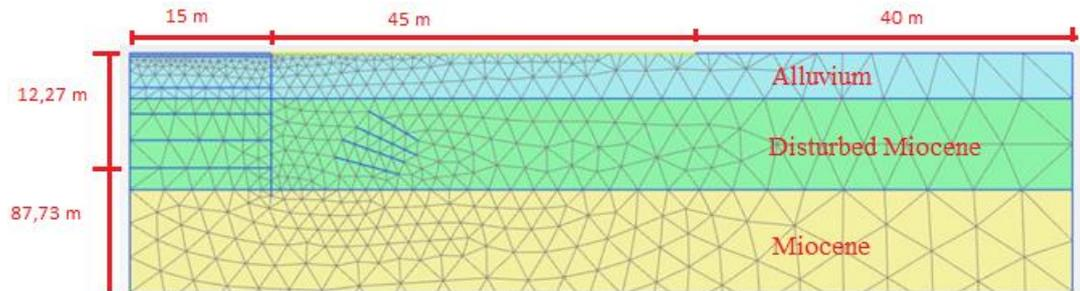
Figure 1. Finite elements mesh adopted
