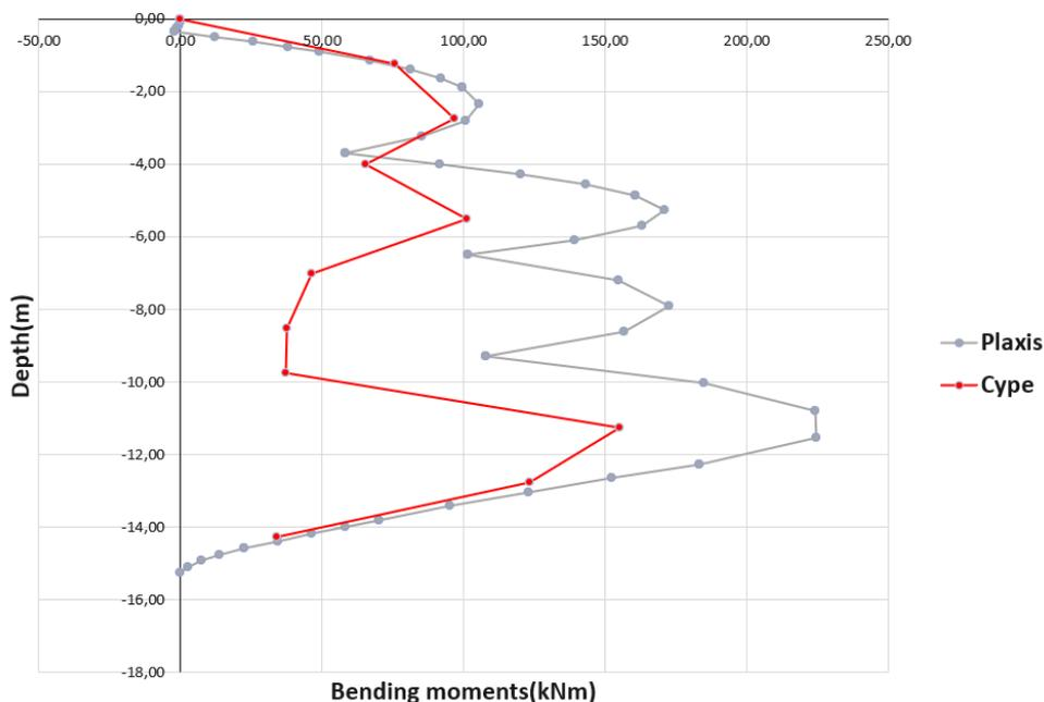
Figure 3. Retaining wall's bending diagram obtained by PLAXIS 2D ® and Cype-StruBIM Embedded Walls
