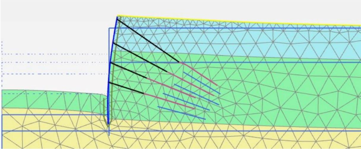
Figure 2. Deformed mesh at the last excavation stage (the full dimension of the model was not presented to zoom the area around the retaining wall)
