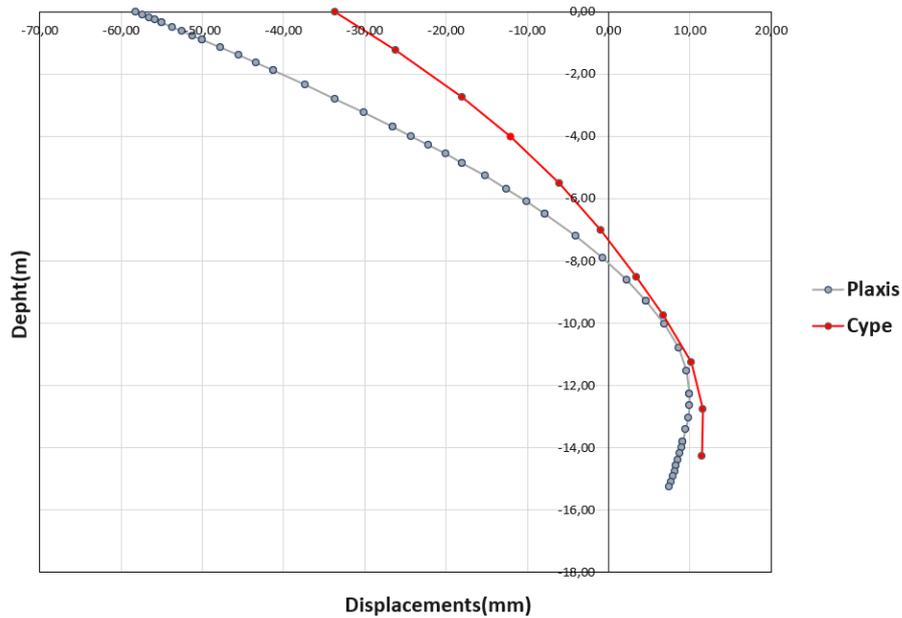
Figure 4. Comparison between PLAXIS 2D ® and Cype-StruBIM Embedded Walls in terms of accumulated horizontal displacement on the wall
