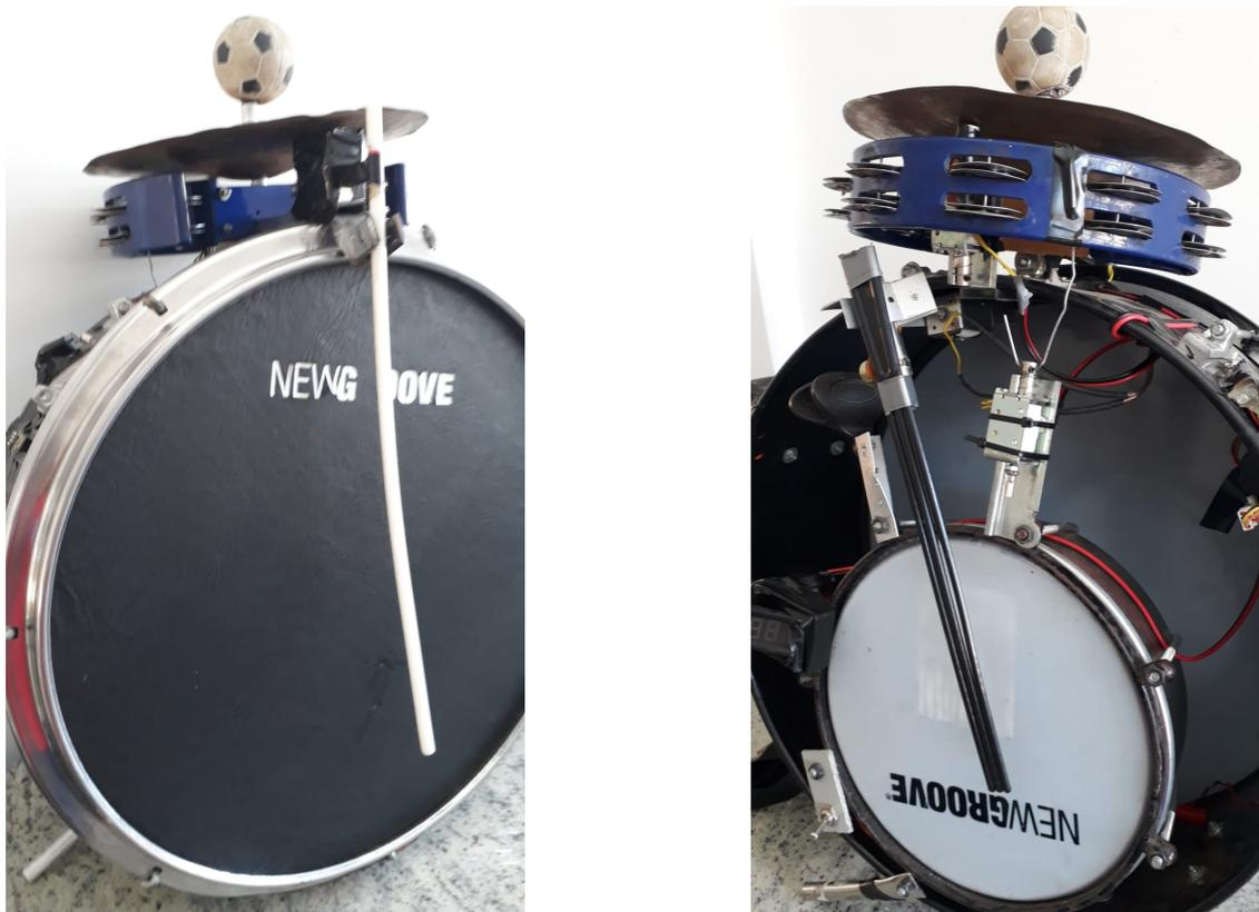
(a) Mechanism of striking the bass drum's side using a nylon drumstick.
