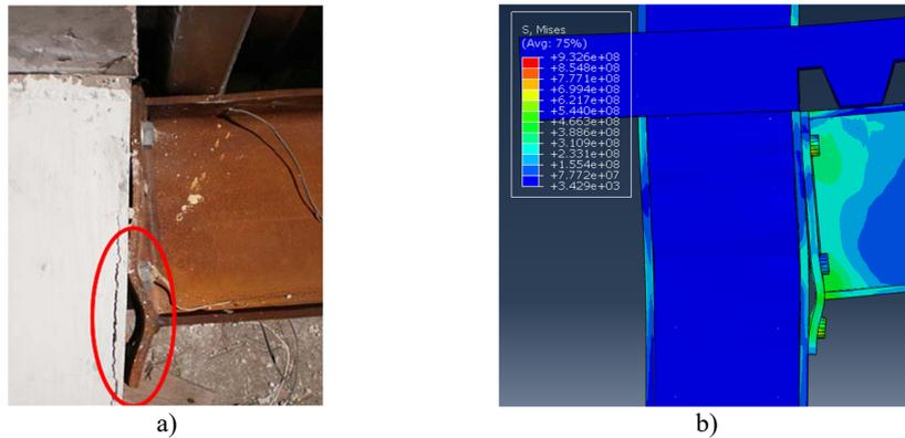
Figure 5 – Deformation of end plate and high-strength bolts a) experimental [9]; b) numerical
