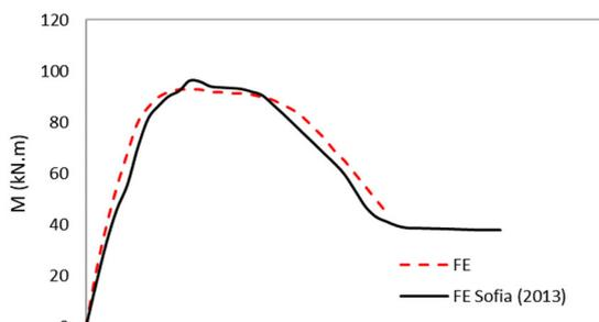
Figure 7 – Moment-rotation behavior of composite joint after fire – comparison with Matias et al [10]
