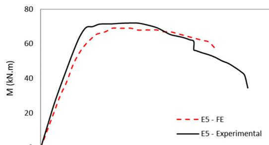
Figure 8 – Moment-rotation behavior of composite joint in E5 test
