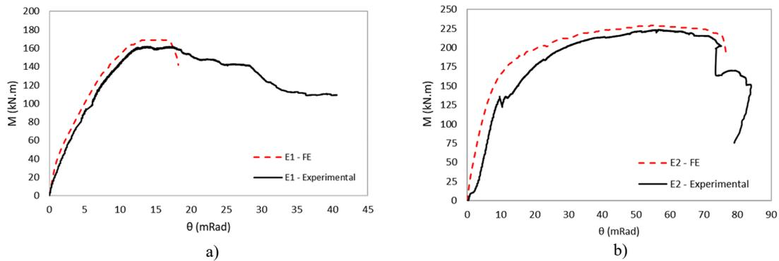
Figure 3 – Moment-rotation behavior of composite joint a) E1 test; b) E2 test.
