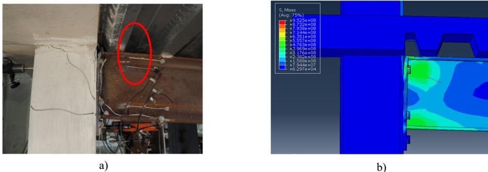
Figure 4 – Deformation of end plate a) experimental [9]; b) numerical
