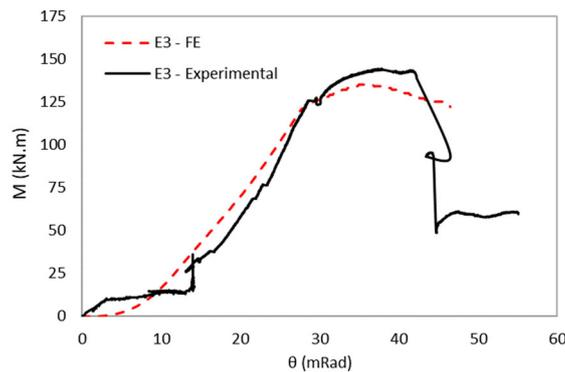
Figure 6 – Moment-rotation behavior of composite joint in E3 test
