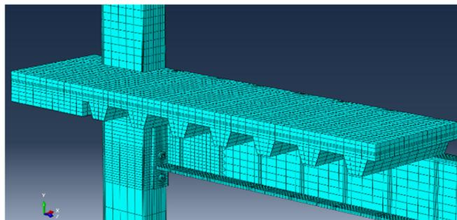
Figure 2. Meshed model for the composite joint
