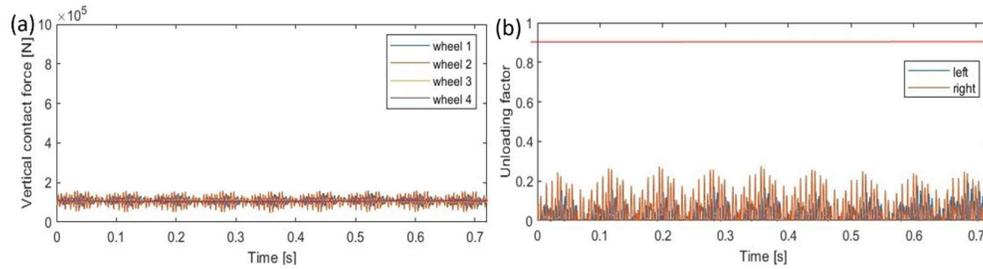
Figure 4 - Time-histories of polygonised wheel: (a) vertical dynamic contact forces and (b) unloading factors (1<sup>st</sup> wheel, right side)
