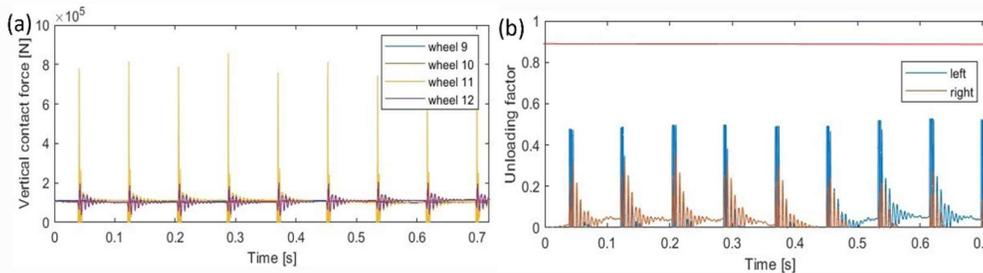
Figure 5 - Time-histories of wheel flat: (a) vertical dynamic contact forces and (b) unloading factors (11<sup>th</sup> wheel, left side)
