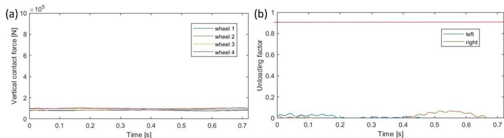
Figure 3 - Time-histories of healthy wheel: (a) vertical dynamic contact forces and (b) unloading factors
