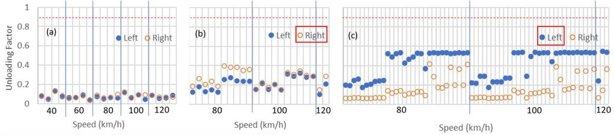
Figure 7 - Influence of the vehicle speed in the unloading factor (a) healthy wheel; (b) polygonised wheel (right side); (c) wheel flat (left side).
