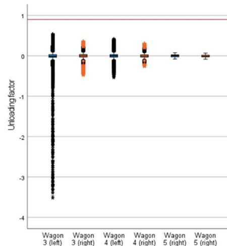
Figure 10 - Boxplots of the unloading factor for the faulty wagon and on the next 2 consecutive wagons - wheel flat (3<sup>rd</sup> wagon, left side)
