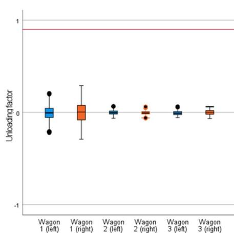
Figure 9 - Boxplots of the unloading factor for the faulty wagon and on the next 2 consecutive wagons - polygonised wheel (1<sup>st</sup> wagon, right side)
