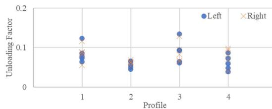
Figure 6 - Influence of the track profile in the unloading factor of a healthy wheel.
