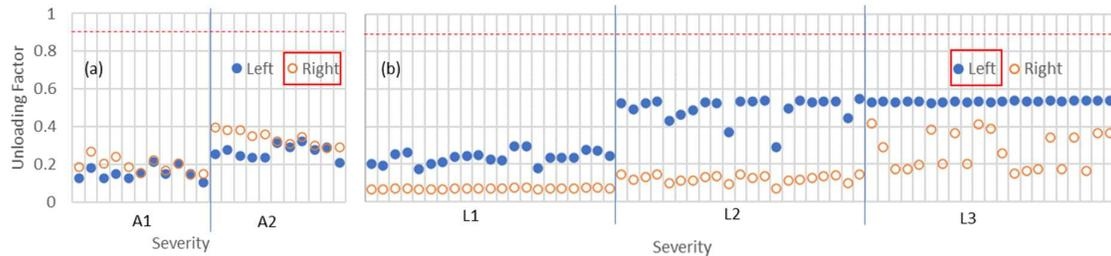
Figure 8 - Influence of the severity of the defect in the unloading factor (a) healthy wheel; (b) polygonised wheel (right side); (c) wheel flat (left side).
