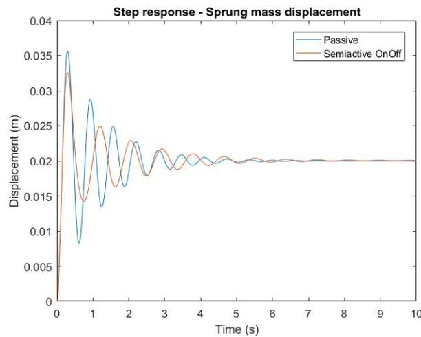
Figure 3 – Time history displacement of the sprung mass
