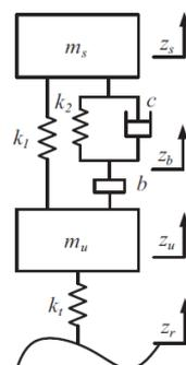
Figure 2 Quarter car model with inerter device [7]
