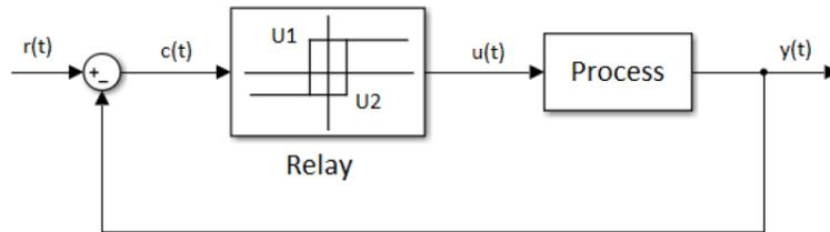
Figure 3 Block diagram of the 'On-Off' control [8]
