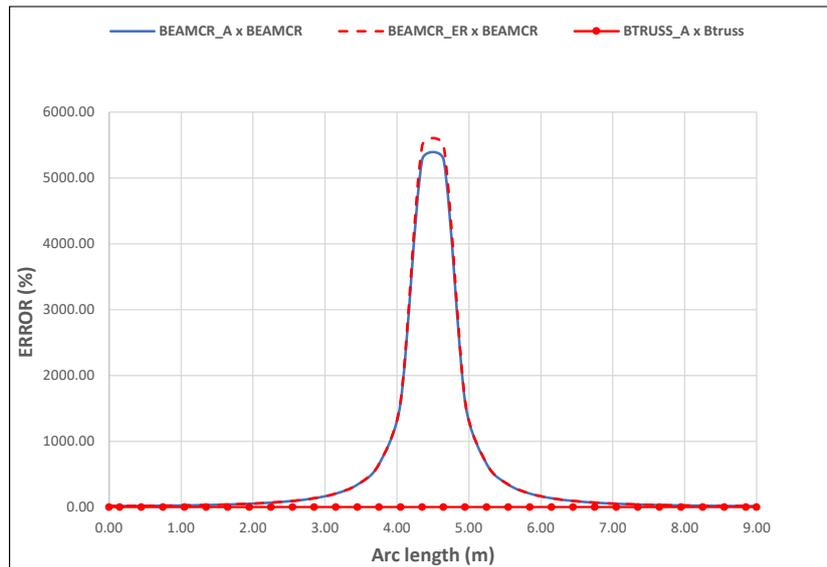
Figure 5. Percentage error between using any alternative (“assembly” or Euler-Rodrigues formula) and not using them
