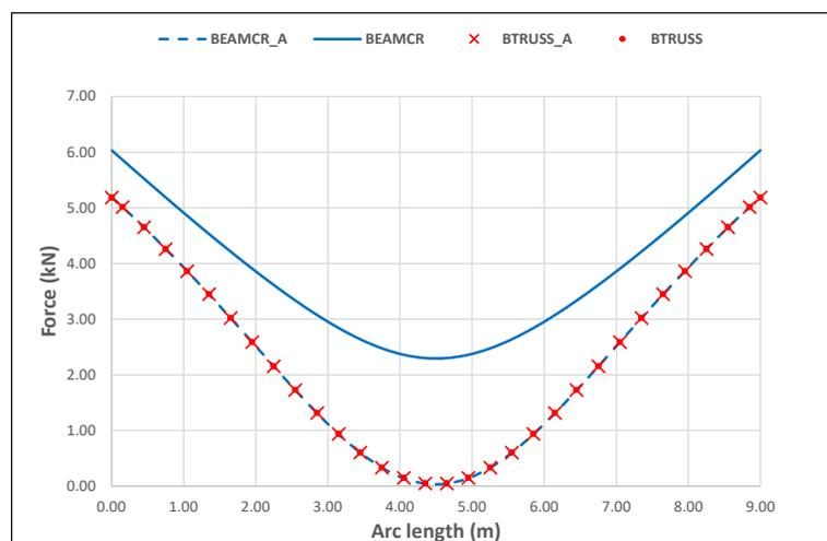
Figure 2. Comparison of the distribution of forces along the element, without using the Euler-Rodrigues formula
