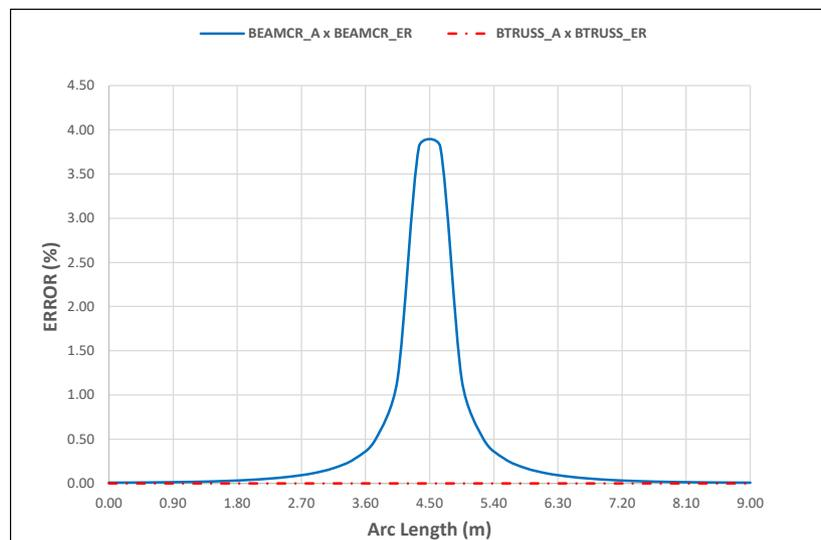
Figure 4. Percentage error between the results of forces along the beam using “assembly” and Euler-Rodrigues formula
