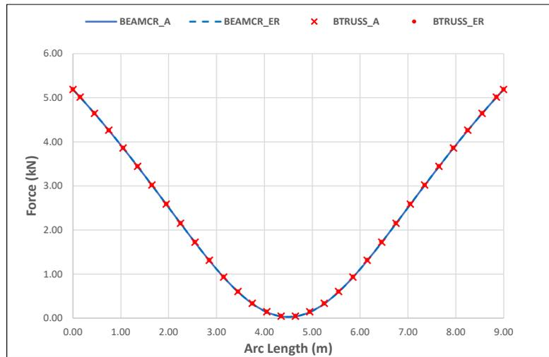
Figure 3 .Comparison of the distribution of forces along the element, without using the Euler-Rodrigues formula
