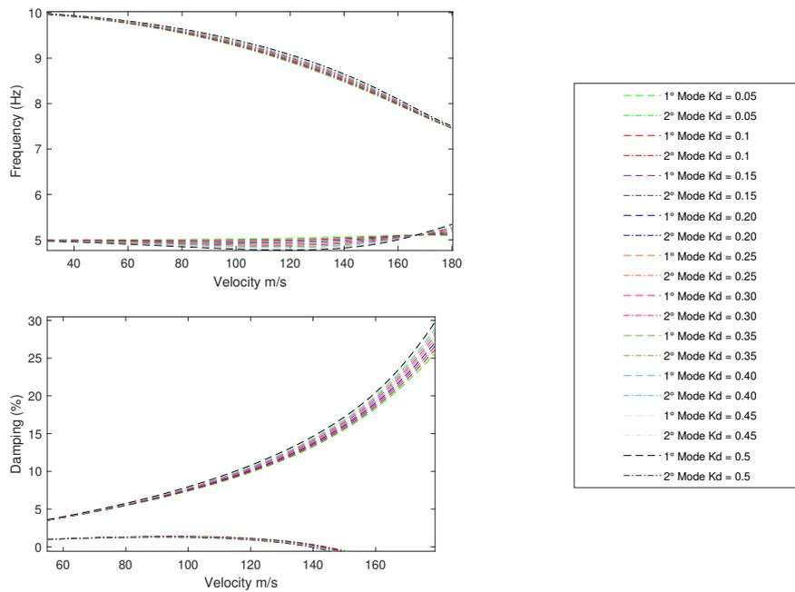
Figure 4. Behavior of the aeroelastic system given the proportional gain variation from the controller
