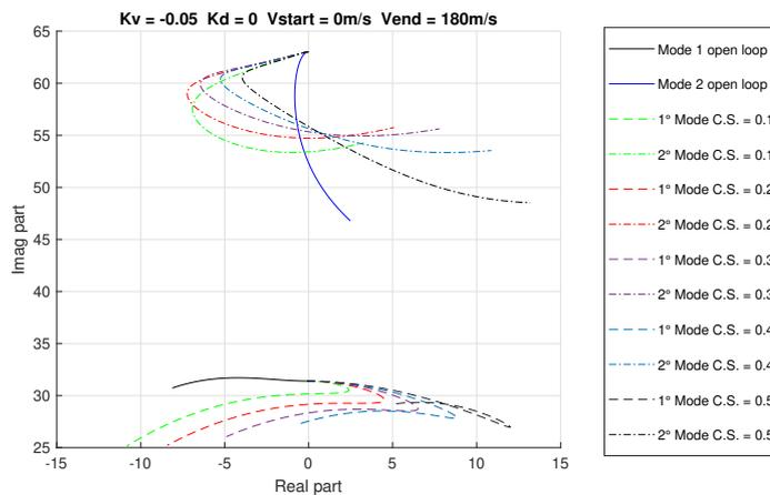
Figure 6. Root locus for open and closed loop.
