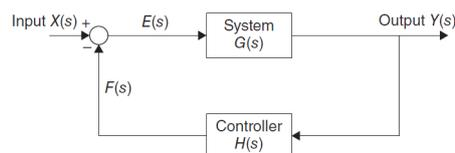
Figure 2. Closed loop system with controller in the feedback loop:[1]
