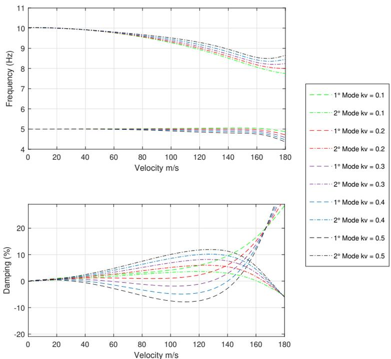
Figure 3. Behavior of the aeroelastic system given the derivative gain variation from the controller
