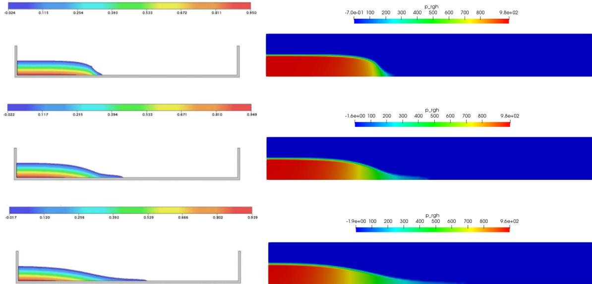
Figure 1. Pressure fields in Freeflow (left) and OpenFOAM (right) through times 0.1, 0.2 and 0.3s
