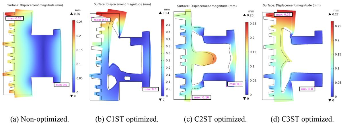
Figure 1. Optimization results: Thermal compensation, total displacement magnitude (8:1 scale).
